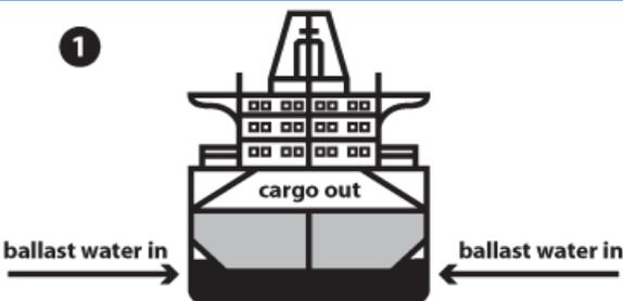
1. At source port, unloading cargo, filling with ballast water (ballasting).
