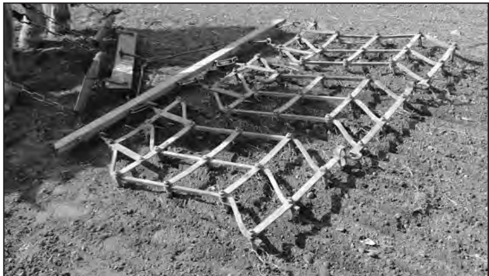
Picture of a spike tooth harrow, the kind Nicholas probably used. Harrowing was done after ploughing to further spread and even out the dirt for planting. The harrow was pulled by horses or oxen. Photo by Ken Giorlando.
