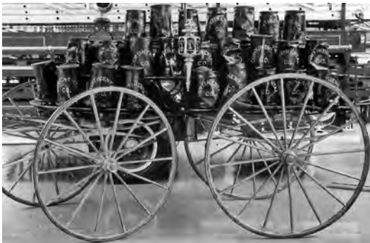
Bucket carriage of unknown make, c.1860, used by Jamaica, Long Island, Continental Bucket Company #1, carries 50 tarred canvas buckets, all of which are inscribed “Continental Company.”
