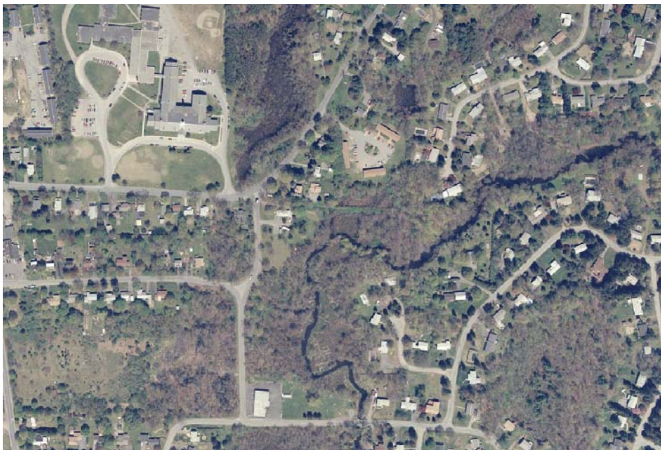
Figure 5. The aerial photo shows the Fall Kill passing through a residential neighborhood between Haviland Road and Roosevelt Road. The area has been prone to flooding and is a suspected source of fecal coliforms because of the use and proximity of septic systems to the creek. (Photo courtesy of DCEMC)
