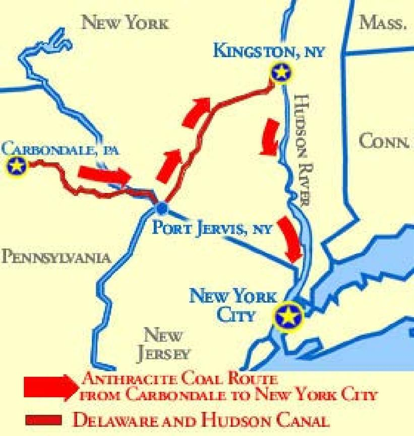
Once complete the canal ran 108 miles long, ending at the city of Kingston. It was 4 feet deep, 32 feet wide and changed a total of 1075 feet in water elevation.
